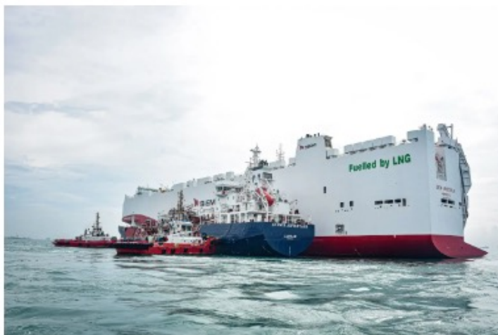
A ship-to-ship Liquefied Natural Gas (LNG) bunkering transfer operation from MV Avenir Advantage, Petronas' first LNG Bunkering Vessel (LBV) to SIEM Aristotle, in Pasir Gudang, Johor, on November 11, 2020. — Picture via FACEBOOK/PETRONAS
